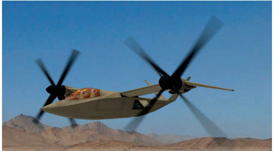
Karem's ATR-36 is the JMR/FVL attack variant, featuring 36 ft (11 m) diameter proprotors that are "very rigid, propeller-like but very light rotor". (All Karem Aircraft graphics)
