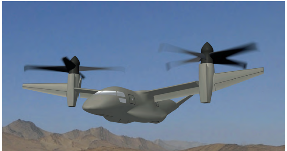
The UTR-36 uses the exact same rotor system and wing mated to a utility fuselage — à la the UH-1 Huey and AH-1 Cobra.
