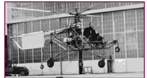
First major configuration of the VS-300 with Serge Gluhareff at the controls undergoing tethered tests at the Vought-Sikorsky hangars, ca. October 1939.
