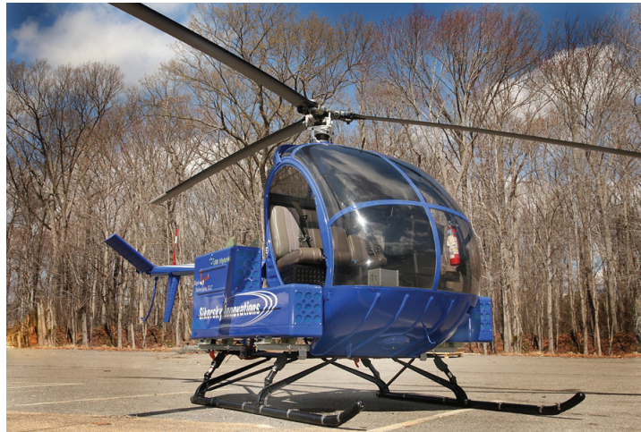
The Sikorsky Firefly integrated a Schweizer S-300C helicopter with all-electric propulsion, but excessively short endurance with battery power stopped the program in 2011 during ground acceptance testing. (Sikorsky Aircraft photo)
