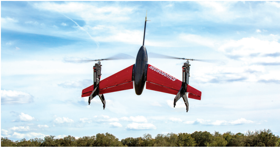
Embry-Riddle University and Heurobotics are collaborating on the all-electric Mark II UAS. The tail-sitting vehicle uses two fully articulated rotors and tips over to transition from vertical takeoff to wing-borne cruising flight. (Heurobotics photo)
