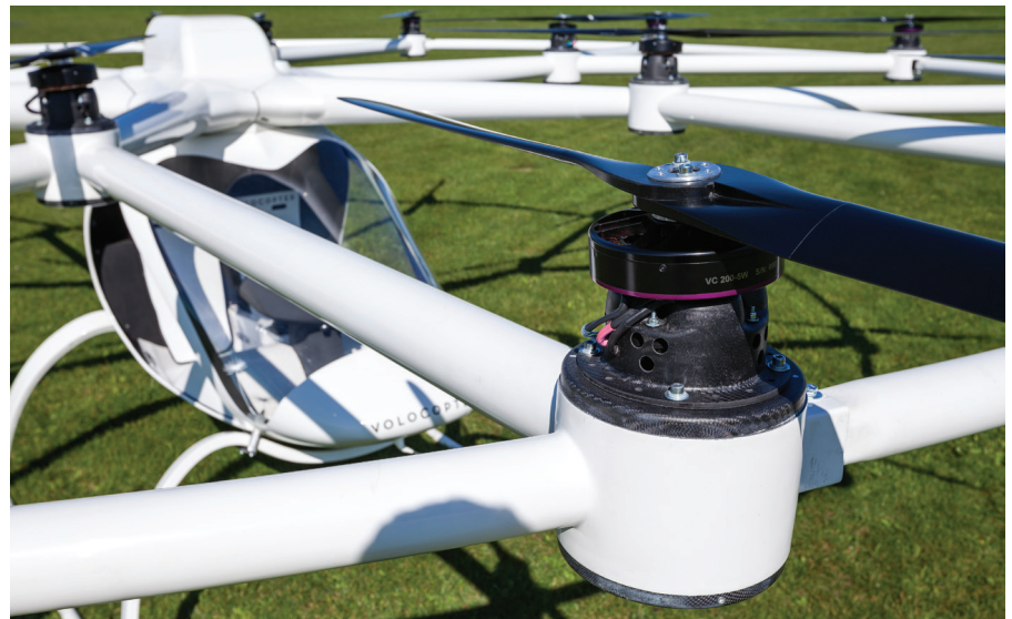
Distributed Electric Power aircraft, like the Volocopter VC200, package drive motors and propellers without a driveshaft to eliminate transmission losses and give designers new flexibility. (e-vo GmbH photo)
