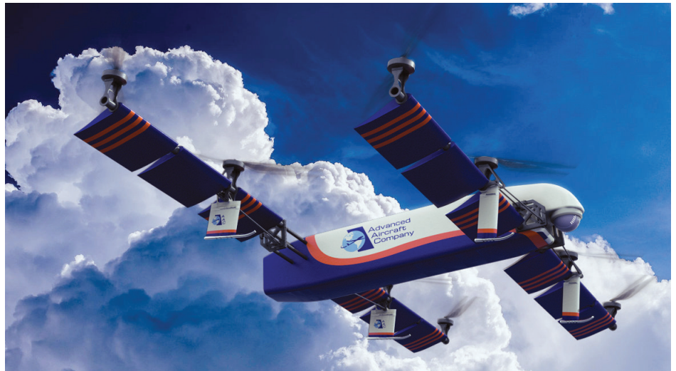
Advanced Aircraft Company is near low rate initial production of the Hercules multi-rotor VTOL UAS with a hybrid gasoline-generator propulsion system. (AAC graphic)
