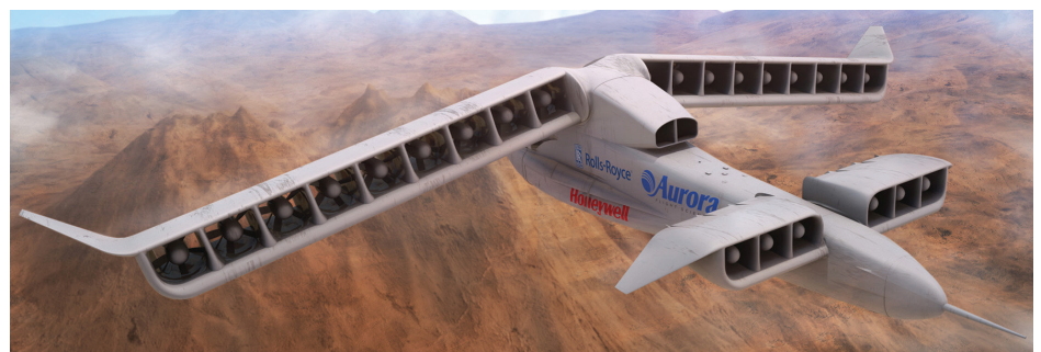
The DARPA LightningStrike VTOL X-Plane designed and built by Aurora Flight Sciences will integrate a Rolls-Royce AE1107C turboshaft with Honeywell megawatt generators to provide hybrid electric power for 24 ducted fans. (Aurora graphic)
