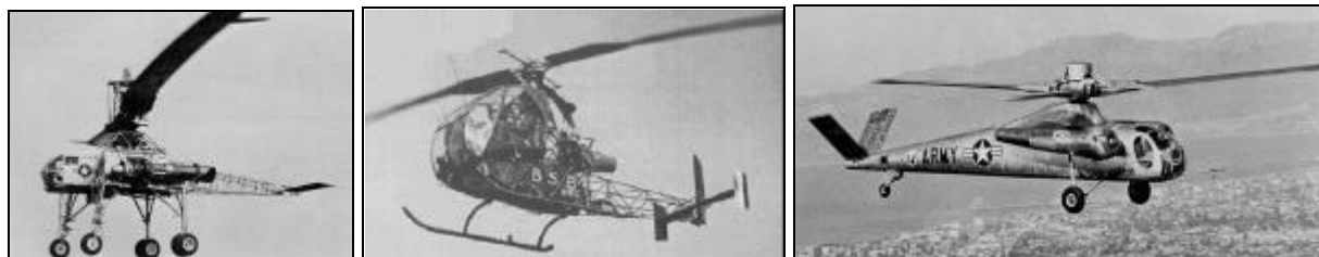
Figure 41. The Hughes XH-17 tip jet helicopter (left), the Sud Aviation Djinn cold cycle helicopter (center), and the Hughes XV-9 hot cycle helicopter (right).
