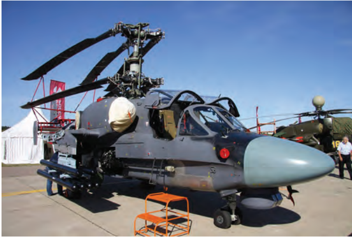
An upgraded version of the carrier-based Kamov Ka-52K helicopter, seen here MAKS 2015 airshow, showing the new EOS-52 EOTS system. (AHS photos by Grigory Omelchenko)
