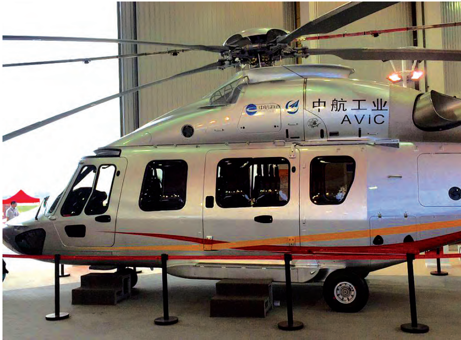
The AC352 is the Avicopter version of the Airbus H175. The primary difference is the use of Chinese avionics and the joint AVIC-Turbomeca engine. (Turbomeca photo)
