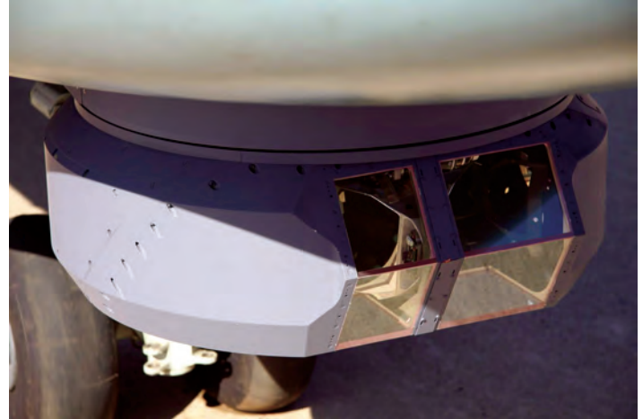
An upgraded version of the carrier-based Kamov Ka-52K helicopter, seen here MAKS 2015 airshow, showing the new EOS-52 EOTS system. (AHS photos by Grigory Omelchenko)
