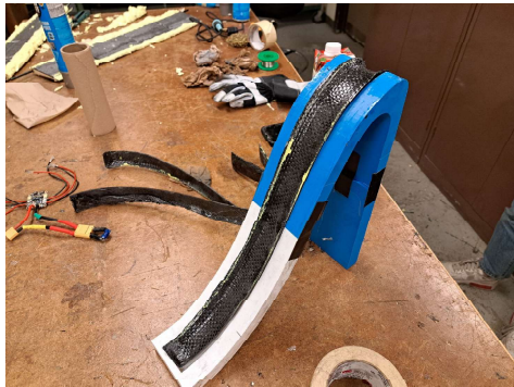
Figure 18: Wet Layup of Landing Gear Using a 3D Printed Mold
