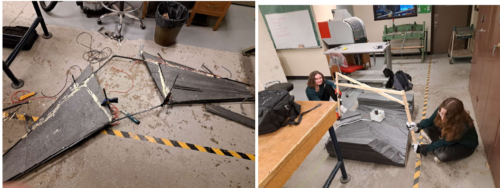
Figure 16 & 17: Wings and Spars Integration & Use of Custom Hot Wire Foam Cutter.
