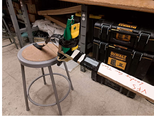
Figure 4: Use of the landing gear test stand to confirm the strength of the landing gear.
