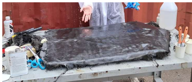
Figure 17: Wet Layup of Fuselage Using a Foam Mold
