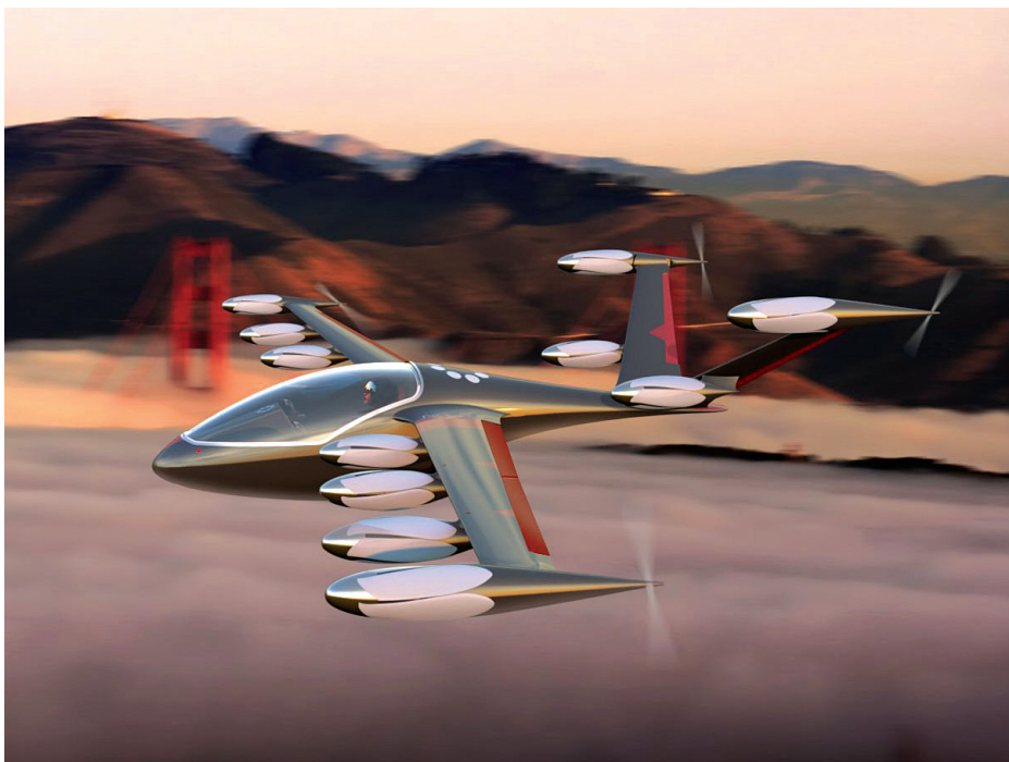
With the VTOL propellers folded back, the S2 cruises on its aerodynamically efficient wing, with thrust provided by four cruise propellers.
