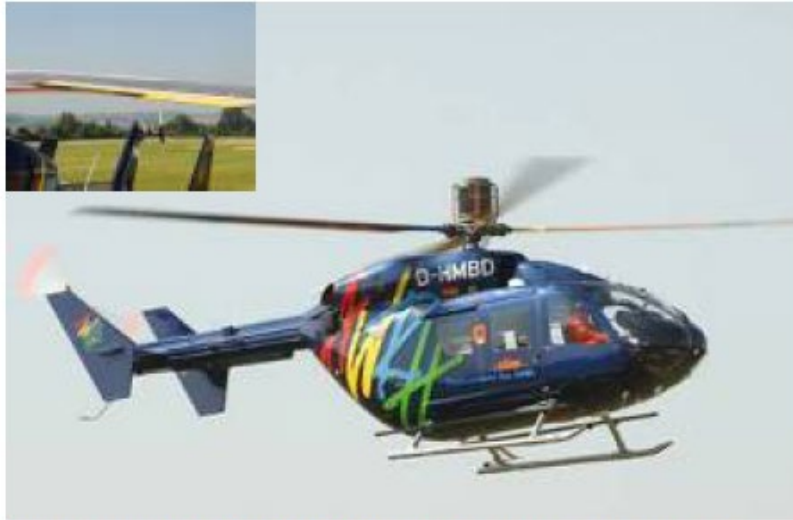
BK117 S7045 with active flaps rotor
