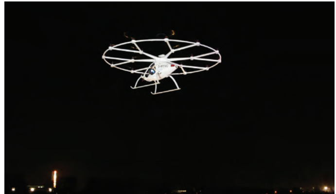
As of early April, the e-volo VC200 Volocopter had made more than 300 flights, including this tethered unmanned nighttime flight. (e-volo photo)
