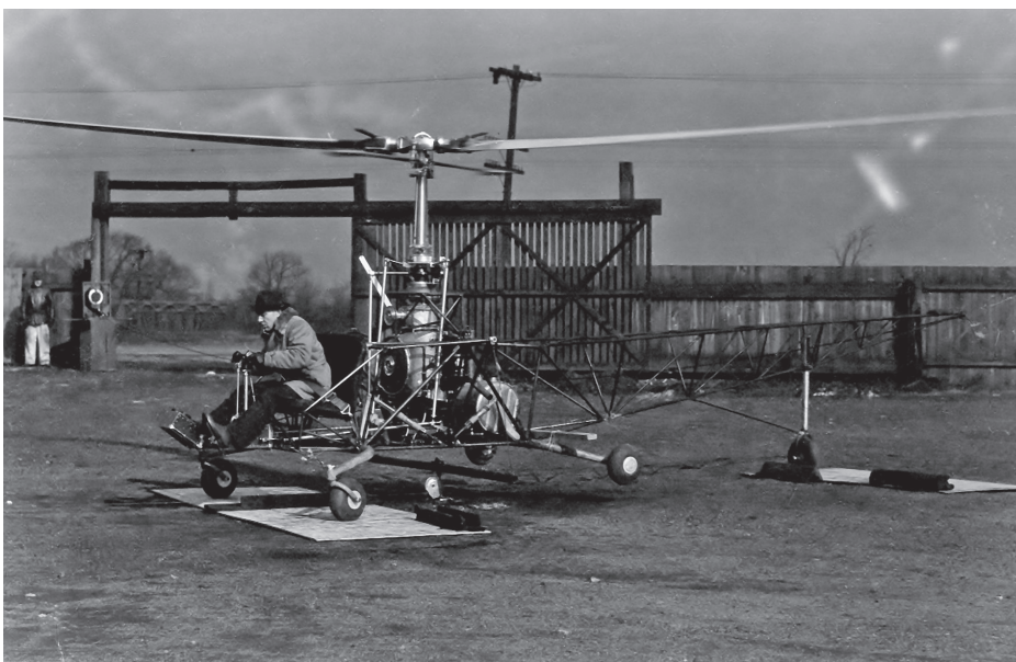
Although the Gardenville team was only formally authorized to build and test two helicopters, they went ahead and built a third based on their experience with the first two. It became the basis for Bell's Model 47, the first civil-certified helicopter.
