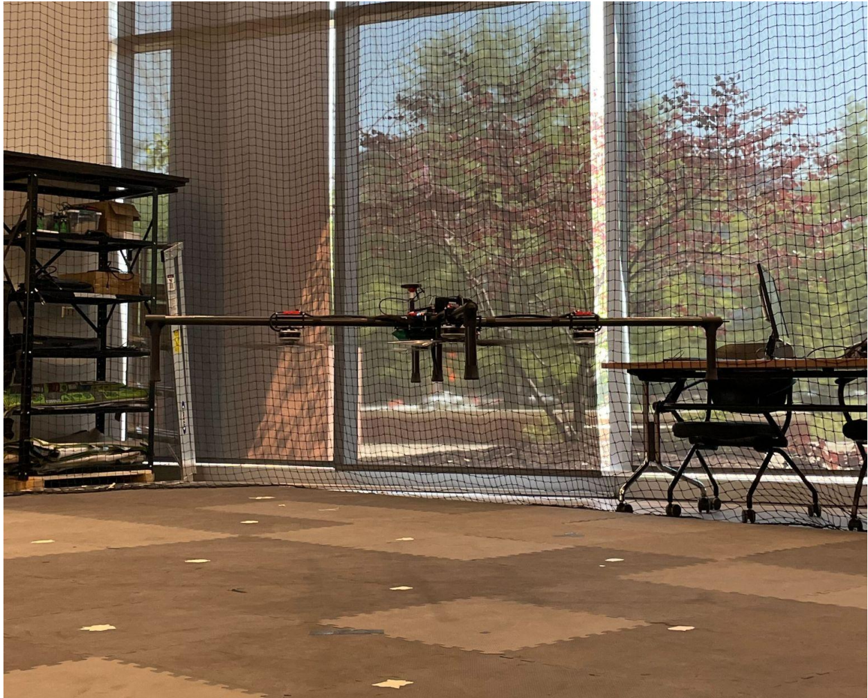
Fig. 21. Hover test of Foxtail without wings in the Brin Family Aerial Robotics Lab.
