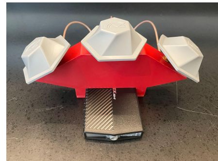
Fig. 20. Upgraded FPV Antennas
