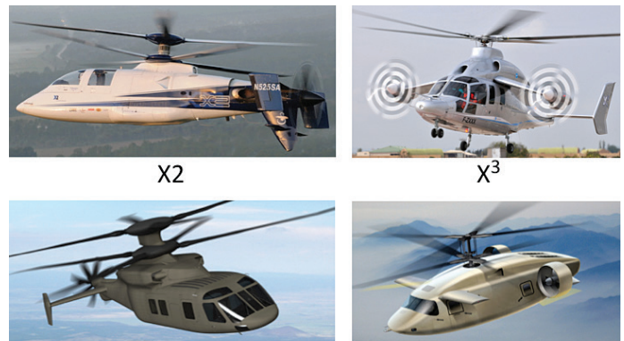
Recent (top) and JMR compounds: Sikorsky X2, Airbus Helicopters X 3 , Sikorsky-Boeing SB>1 and AVX compound aircraft.
