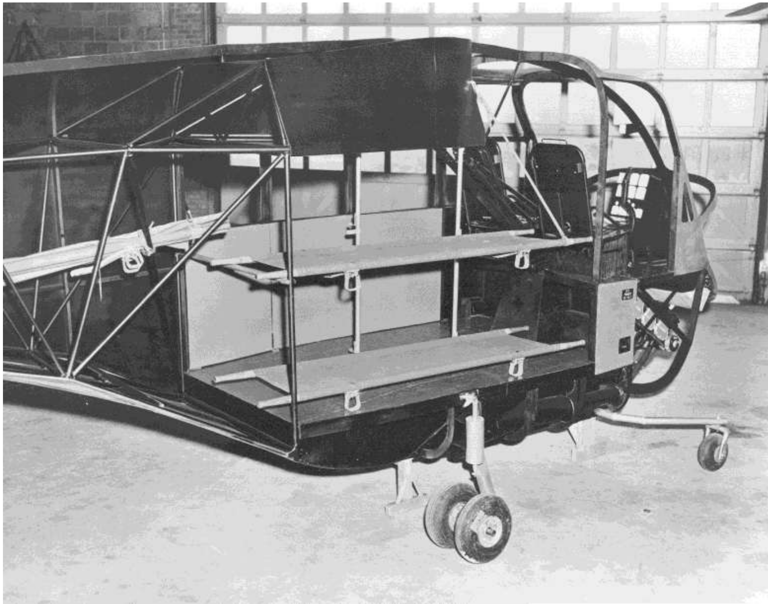
LZ-5 mockup with stretchers for showing to U.S. Army Medical Corps. Picture and article published in Aviation Week, January 7, 1952
