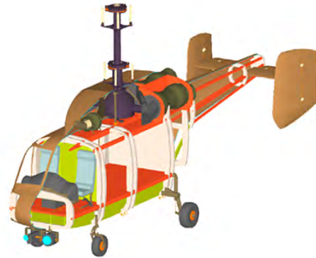
Figure 4.14: Figure showing the structure of the airframe.
