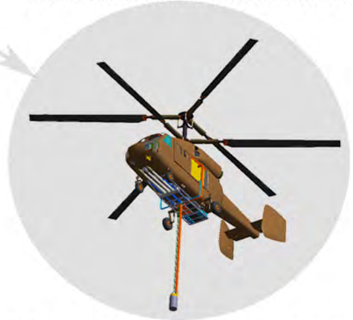
Self Contained Firefighting Module
