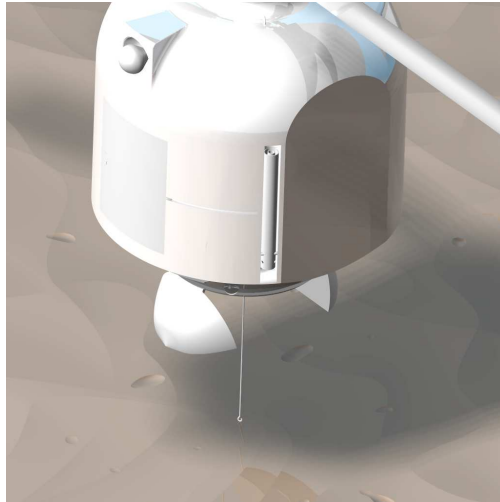
Figure 2.27: Bottom door open, hoisting cable loose
