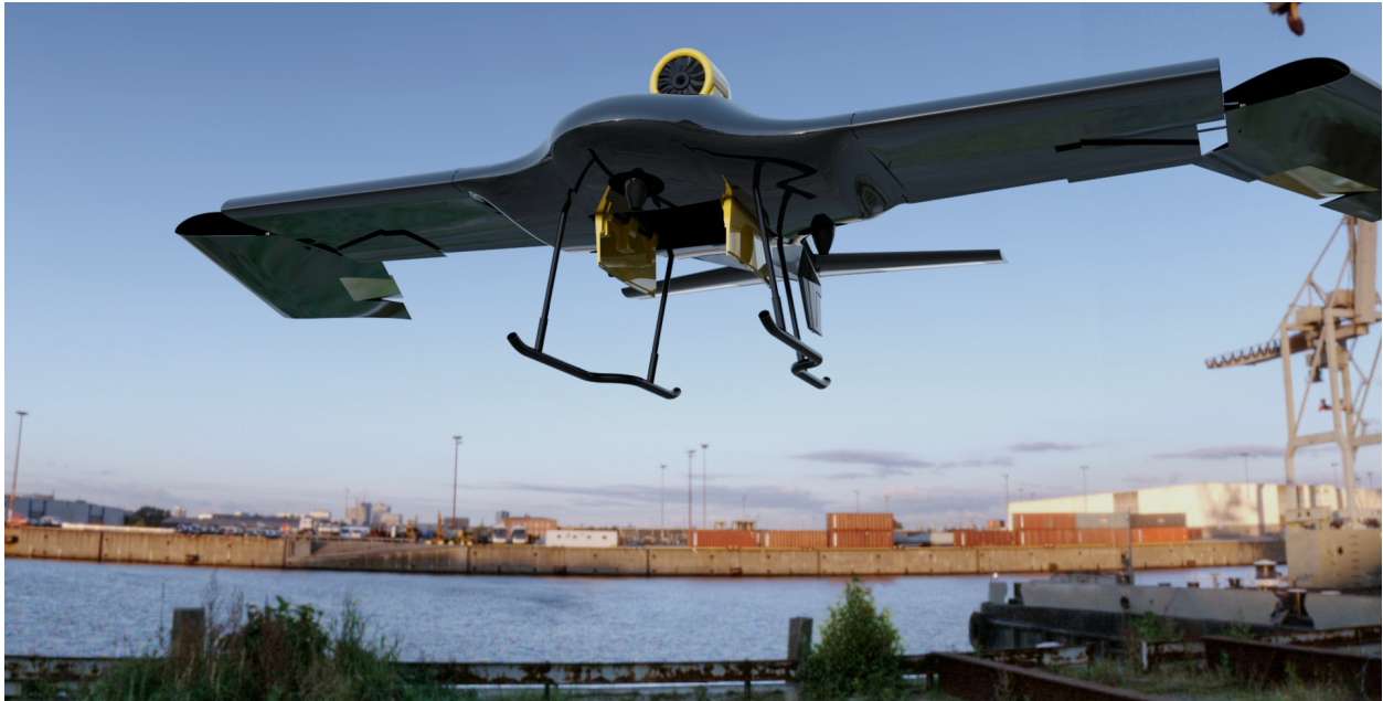
Figure 8: The New River Harrier in hover with wings folded back. Note the moveable panels in their retracted position on the underside of the inner wings.
