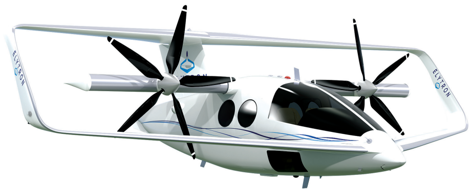
The 4S is a four-seat model under development. The box wing/tilt wing should facilitate excellent STOL capabilities, in addition to vertical flight. (Elytron)
