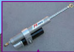
Electro-Hydraulic Actuator M-Mac "MM-15" 12" Stroke Length 100-2,200 lbs Bi-directional 12-24V Supply
