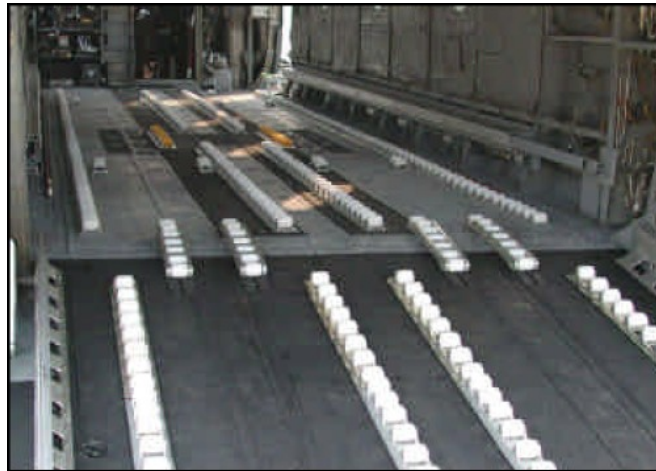
Figure 30: Chinook cargo handling system (DRST, 2005)
