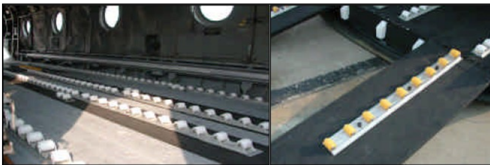
Figure 31: Flip-over roller system (DRST, 2005)
