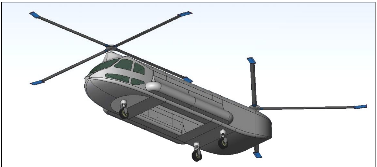
Figure 41: Cargo bay, showing the open floor design, allowing for quick payload release
