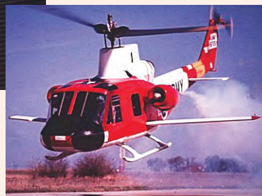
The Bell Model 533 reached an incredible 316 mph in 1969. It was tested with various combinations of rotors, wings and jets, including a winged 2-bladed version (right) and a 4-bladed version with the engines mounted on stub wings (above).
