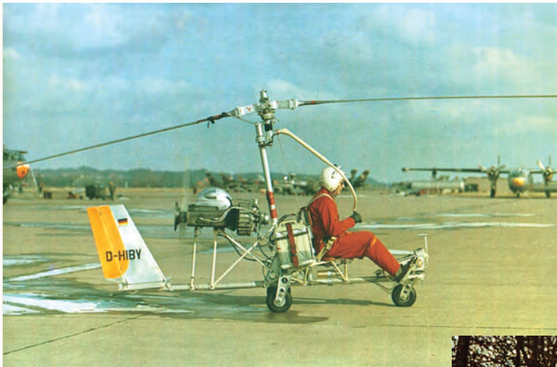
Although it resembled a typical autogyro, the VFW H2 was able to takeoff and land vertically, as well as hover.
