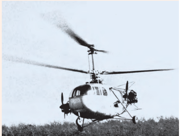
The Gyrodyne GCA-2A was the first compound to fly in the US. It added two propellers on the side of a standard Bendix Model J helicopter.
