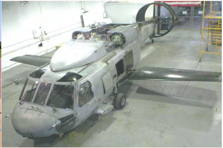
Piasecki has updated their Ring-Tail concept as the Vectored Thrust Ducted Propeller (VTDP), being fitted to a YSH-60F Seahawk, dubbed the X-49.
