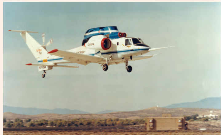
The Sikorsky S-72X, seen here in fixed-wing configuration, was intended to test the innovative X-Wing, but was never utilized for this purpose.
