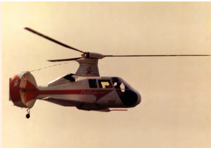
Piasecki pioneered the Ring-Tail on its 16H-1 Pathfinder as a means of auxiliary propulsion and anti-torque control.
