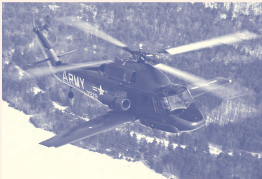
Along with an auxiliary turbojet, Kaman's UH-2 Compound Seasprite flew with the wings of a Beech Queen Air to offload the main rotor in high-speed flight.
