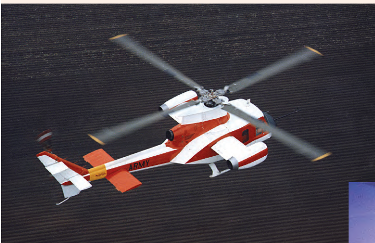
The Bell Model 533 reached an incredible 316 mph in 1969. It was tested with various combinations of rotors, wings and jets, including a winged 2-bladed version (right) and a 4-bladed version with the engines mounted on stub wings (above).
