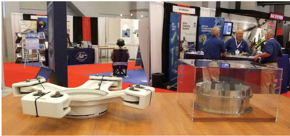
The computer-controlled HMVS active vibration management solution (right) puts counter-rotating masses near the main rotor in place of a heavy, passive bifilar (left). (AHS photo)
