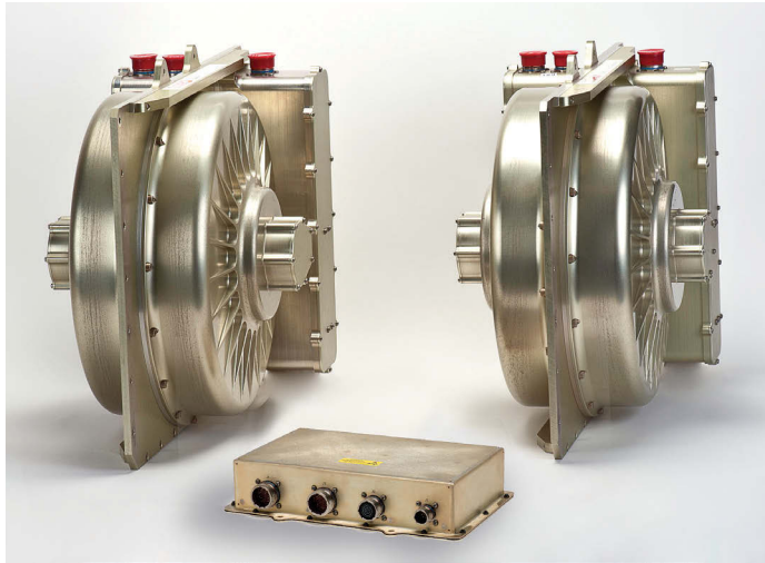
Circular Force Generators (CFG) are a more effective type of Active Vibration Control System (AVCS) particularly suited for medium and larger rotorcraft. (LORD photo)
