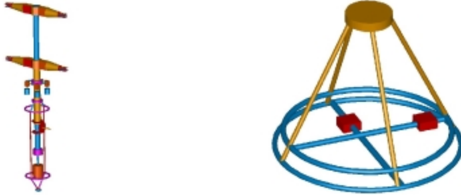
Figure 13.2: Control by shaft tilt and CG shift
