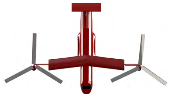
Top-Down view of HealCopter, highlighting 7 foot tilting portion of each wing
