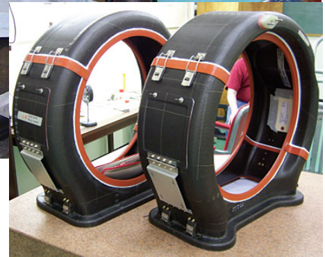
Eagle Technologies designed, prototyped, tested and now manufactures the S-76D inlet (above) and inlet plenum. (Eagle photo)
