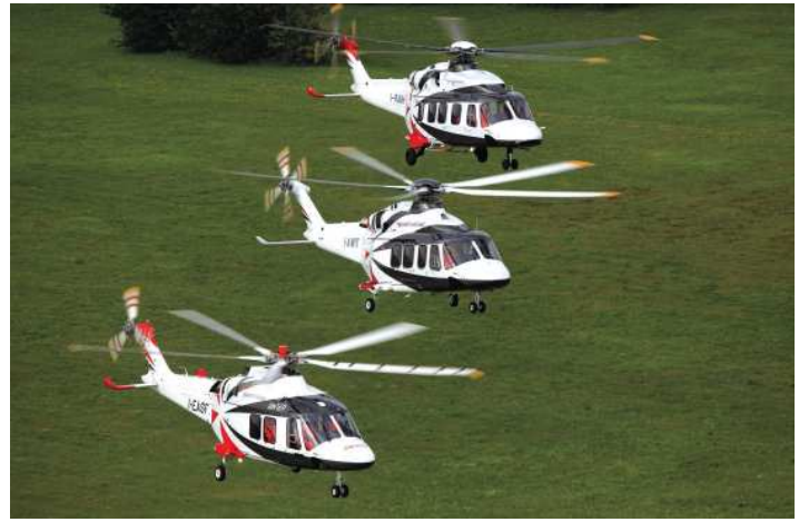
AgustaWestland's family of new aircraft – (left to right) the AW169, AW139 and AW189 – feature 5-bladed rotors for reduced blade loading and noise generation. (AgustaWestland photo.)
