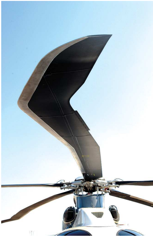
Eurocopter flight tested the Blue Edge blade on an EC155 Demonstrator in 2007. The approach reduces noise generated from Blade-Vortex Interaction. (Eurocopter photo.)
