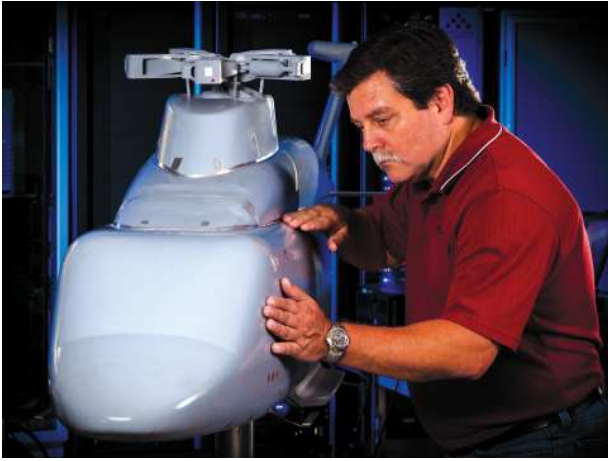
Bell plans first flight of the 525 Relentless next year. It uses a 5-bladed rotor with advanced airfoils and blade tips for reduced noise. (Bell Helicopter photo.)
