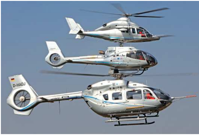
Eurocopter's Fenestron – shown here on the EC145T2 and EC130T2 – has a significant reduction in tail rotor noise in many flight regimes. The experimental X3 removed the tail rotor altogether. (Eurocopter photo by Anthony Pecchi.)
