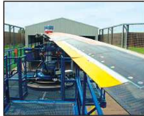
Eurocopter's Blue Pulse active rotor, using piezo-driven flaps on the trailing edge, reduces both external noise and passenger vibrations. Eurocopter began flights in 2005, showing a noise reduction of up to 5 dB. Other manufacturers have ground tested active flaps. (Eurocopter photo)
