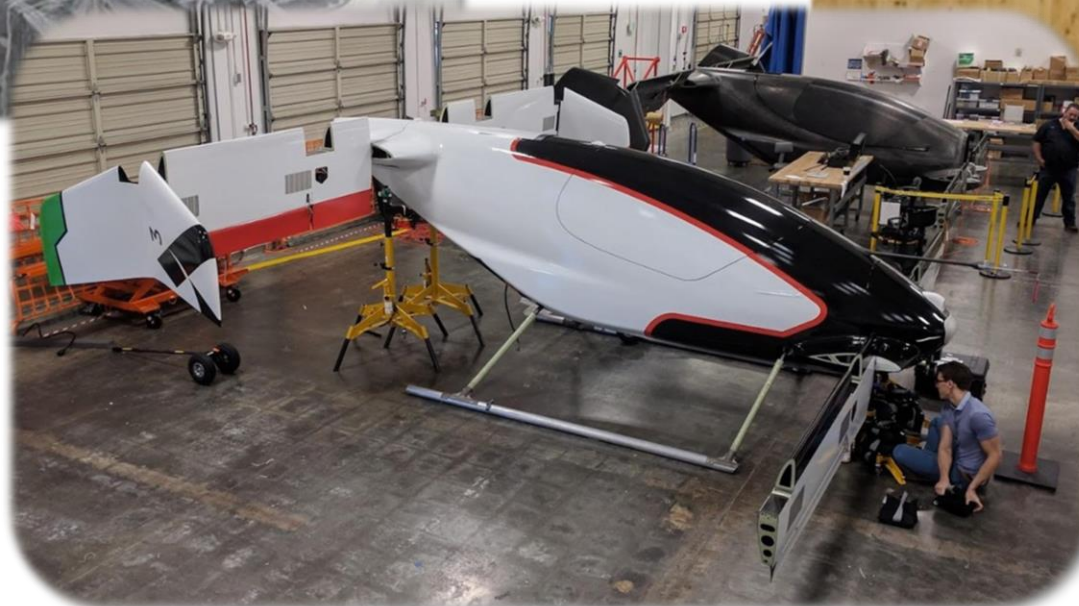
Two full-scale single-seat aircraft under construction
