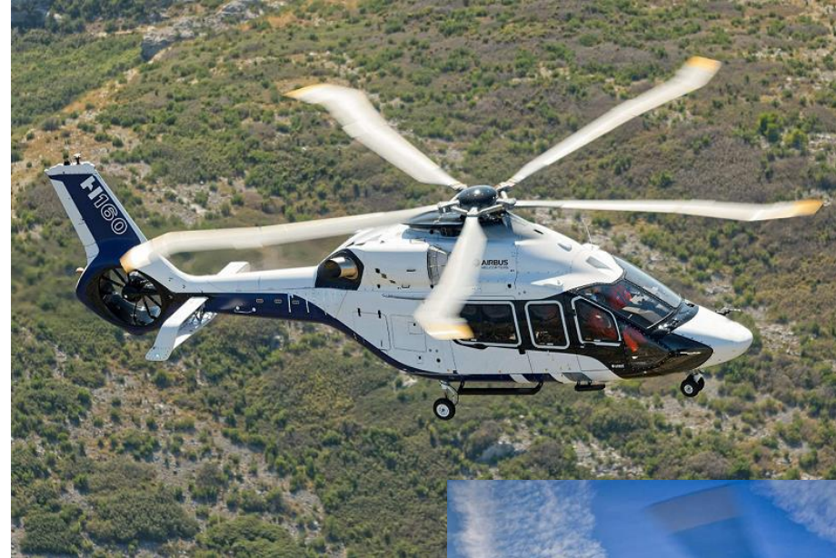
Airbus H160 with Blue Edge Blades and improved Fenestron
