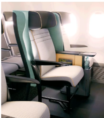
Figure 7: PRM seat extended for use of a passenger without a wheelchair.
