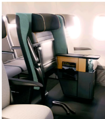
Figure 8: PRM seat folded for use of a passenger with a wheelchair.
