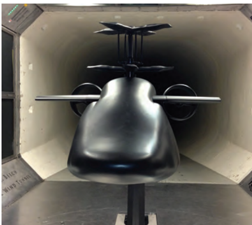
AVX conducted small-scale wind tunnel tests at the National Institute for Aviation Research (NIAR) at Wichita State University. A 1/10th-scale model will run in the low-speed tunnel at Texas A&M early in 2016 under the JMR contract with the Army. (AVX)
